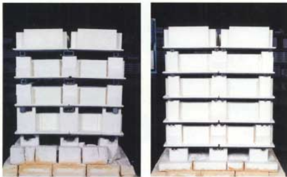
Figure 1. The higher strength of the new beams allowed for the redesign of the kiln cars using thinner beam cross sections of 1/2 in. (right) to replace the existing 1 1/2 in. beams (left).
