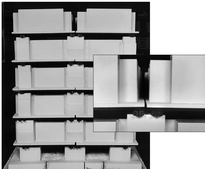
After Retrofit 5 decks with conventional 1/2" Hexoloy SE beams
