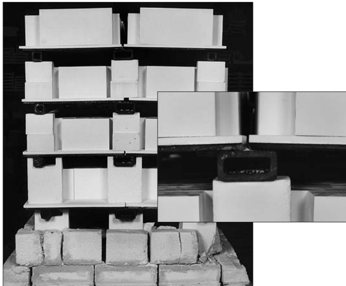
Before Retrofit 4 decks with conventional 1-1/2" beams
